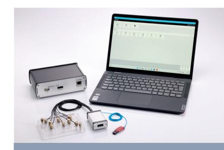
Temperature verification with a multi-probe system allows fast and reliable assessment of the cycler's performance. The generated certificates can support instrument qualification for your quality management system.
