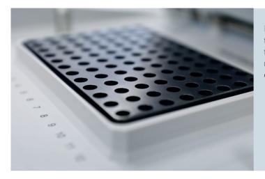
PCR should be faster. That gives you quicker results, throughout the day, and a faster transition to optimal temperatures. The Mastercycler X50 heats with max. 10 °C/s and cools with max. 5 °C/s. Make the speed of the Mastercycler X50 your research advantage.
